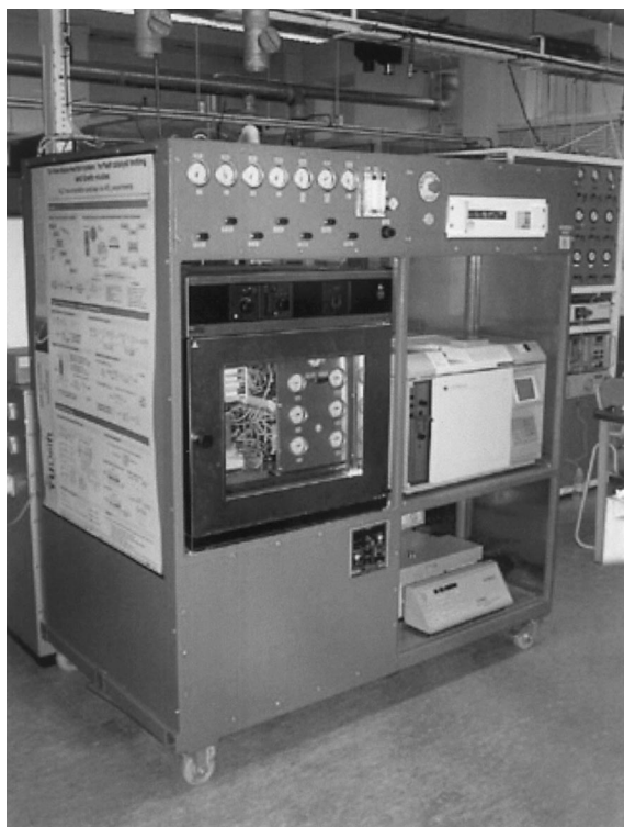
Fig. 5. Photograph of the six-flow reactor set-up for nitrogen oxides ( \text{NO}_x – \text{N}_2\text{O} ) removal.
